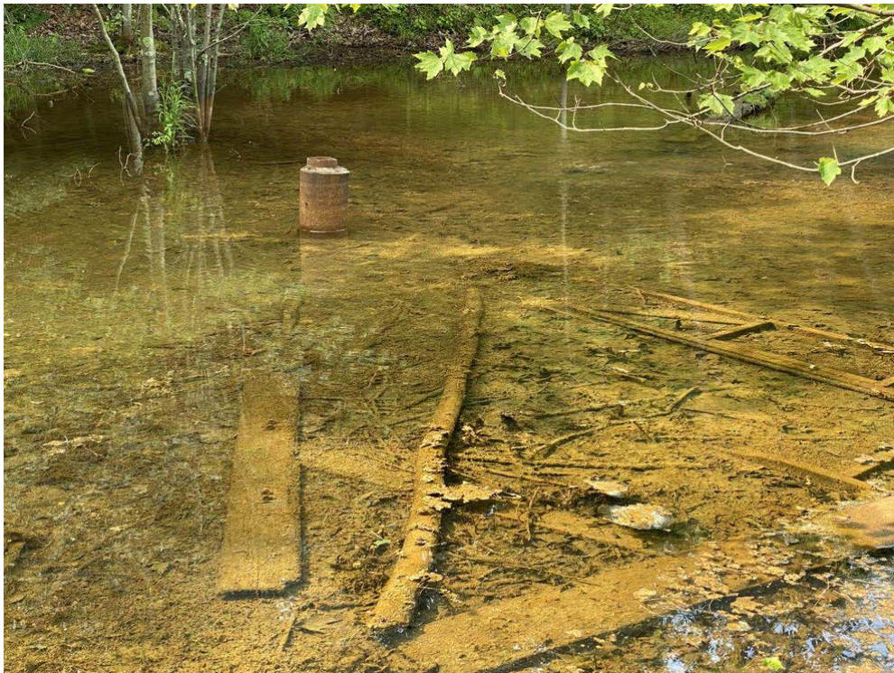
Figure 5-18: E41190747603972 "Pond A Old AMD TS" looking at one of the boreholes discharging AMD from the mine pool
