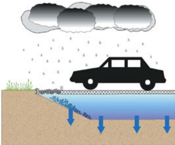
Figure 3. Shows porous pavement and the ability for the stone bed to hold stormwater
