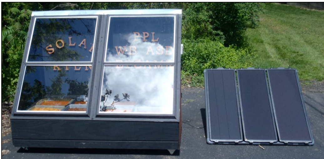
45 Watt Solar Panel Kit (right) powering the EPCAMR Solar AMD Kiln that will be used to dry iron oxide
