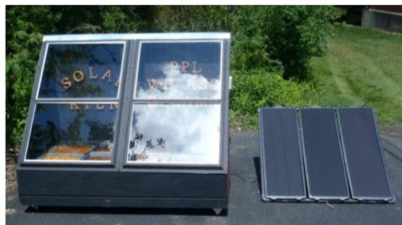
*Fully operational Solar AMD Kiln (left) with 45 Watt Solar Panel Kit (right) powering a ventilation fan*
