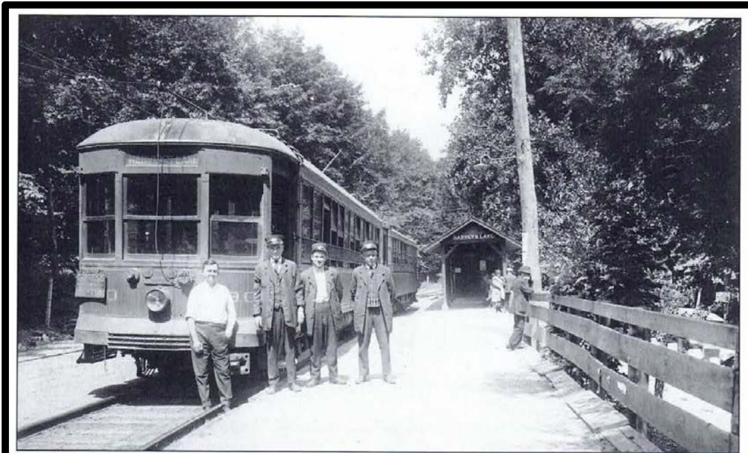
EXPRESS TROLLEY NO. 380 AT THE TROLLEY STATION, 1920s. This photograph includes, from left to right, trolley operators Mr. Keithline, Charles Reid, and Johnson Van Buren Coolbaugh. It shows two trolleys connected by Tomlinson couplers forming a doubleheader to accommodate more passengers. Doubleheaders were prone to accidents. Both trolleys were delivered to the Wilkes-Barre Railway Corporation in 1913. (Courtesy of Joan Coolbaugh Britt.)
