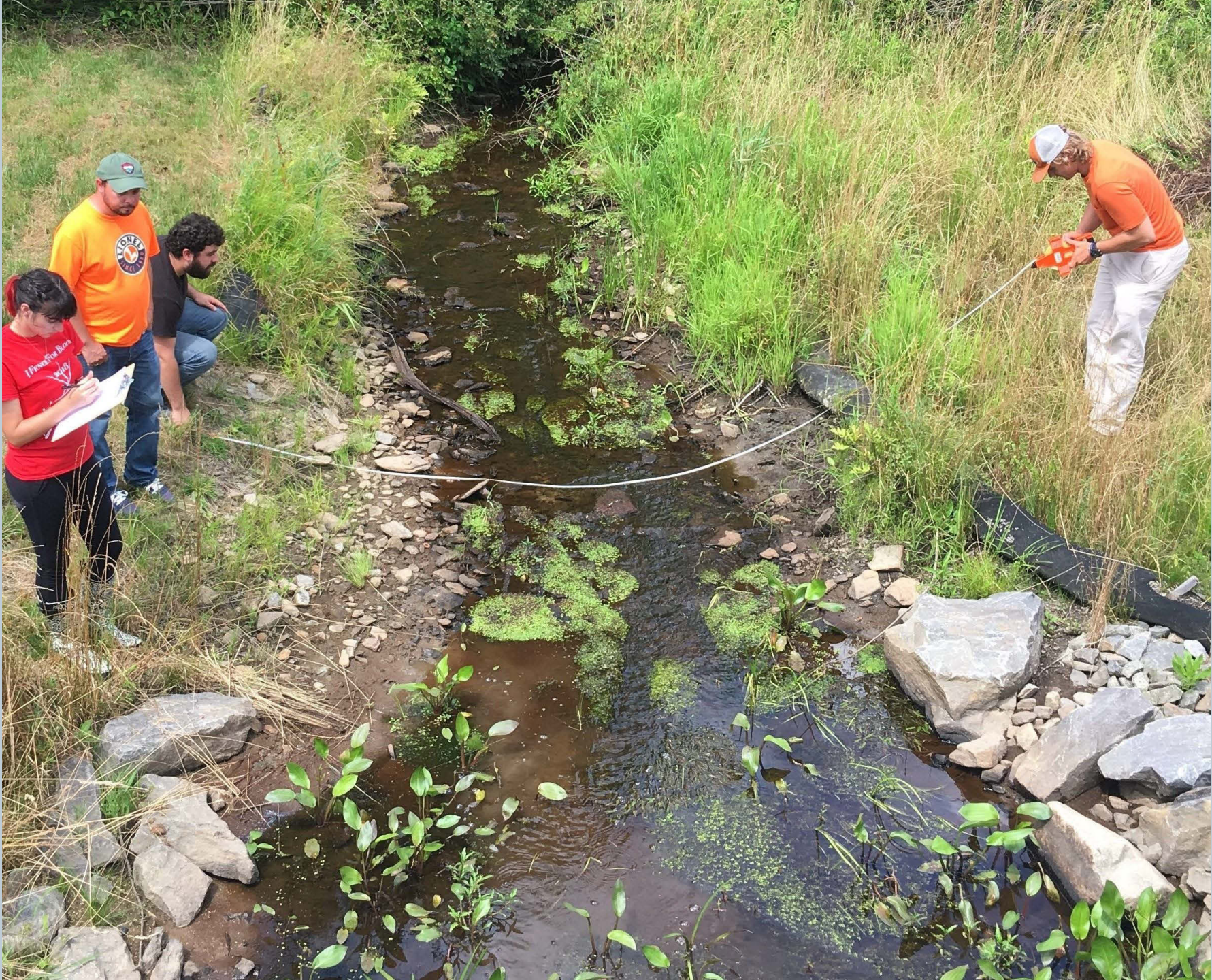
Figure 228. EPCAMR Staff and interns taking Aquatic Organism Passage and culvert measurements of the estimated bankfull width of the unnamed tributary to Toby Creek above the bridge on Hildebrandt Road.
